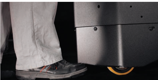
The P-series' low skirt protects the operator's feet without impeding access to ramps and gradients
