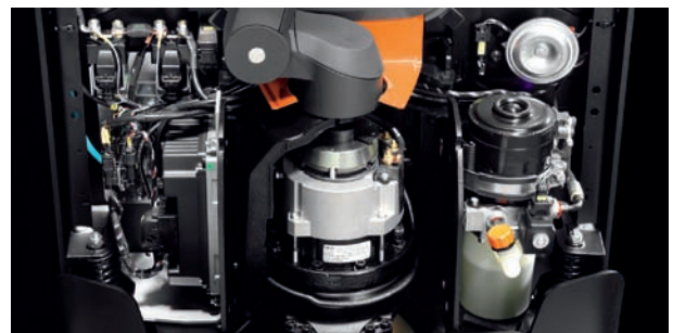
The fixed motor has no moving cables
